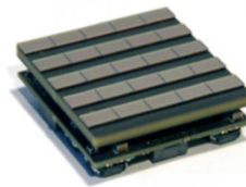
Front side: Tile of the first generation SPADnet sensor
